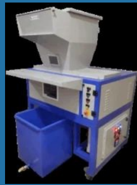
Pouches Shredding And Separation Of Liquid Machine
